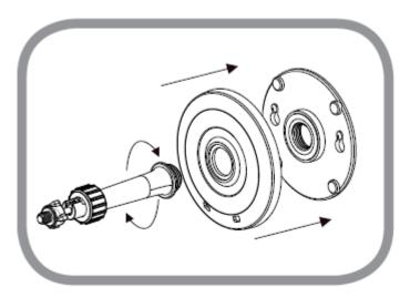
Step 3: Loosen the collar on the camera stem and then screw the camera stem into the bottom of the camera. Turn the securing wheel to ensure the connection to the camera is snug.
