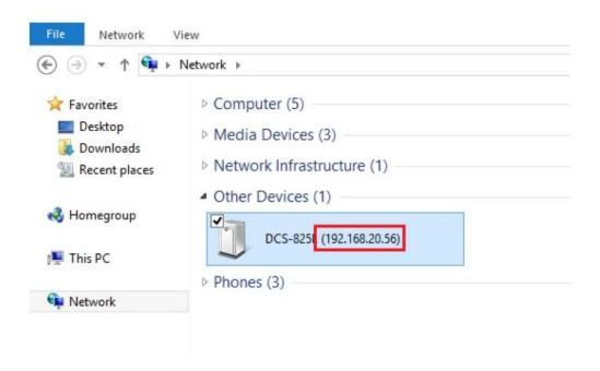
Step 4: Open a web browser and enter "http://IP\_Address/eng/admin/tools\_firmware.cgi" in the address bar (where **IP\_Address** is the IP address you made a note of in Step 3). eg: http://192.168.20.56/eng/admin/tools\_firmware.cgi
