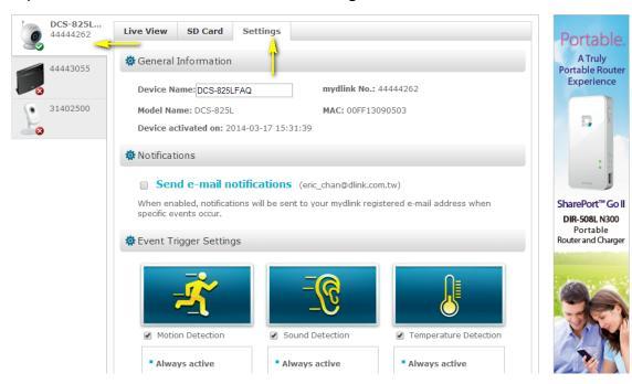
Step 4: Ensure that the Sound Detection checkbox is checked and click the icon.
