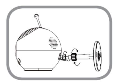
Step 4: Adjust the angle of the camera as desired and then tighten the collar on the camera stem to lock it in place.
